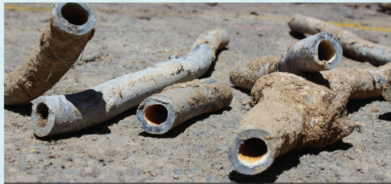
Since its Lead Reduction Program started in 2020, Denver Water has replaced more than 21,000 customer-owned lead service lines with lead-free copper lines at no direct cost to the customer. (Photo: Denver Water)
